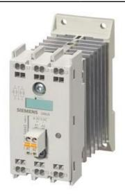
SEMI-CONDUCTOR CONTAC.3-PH.3RF2 AC51 10A 40 DEG. C 48-600V / 230V AC 2-PHASE CONTROLLED SPRING-LOADED CONNECTION BLOCKING VOLTAGE 1200V
