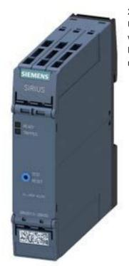
Thermistor motor prot. relay Standard evaluation unit 22.5 mm enclosure Spring-type terminals 2 CO contacts US = 24-240 V AC/DC Manual/Auto/Remote RESET with ATEX certification 2 LEDs (READY/TRIPPED) Protective separation Test/Reset button Open-circuit monitoring Short-circuit monitoring Non-volatile
