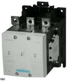
VAC. CONTACTOR, 110KW/400V/AC-3 WITHOUT COIL AUXILIARY CONTACTS 2NO+2NC 3-POLE, SIZE S10 RAIL CONNECTIONS
