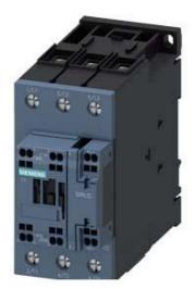
RAIL-CONTACTOR, AC-3, 18.5KW/400V, 1NO+1NC, 110VDC, 0.7...1.25\*US, WITH VARISTOR, 3-POLE, SIZE S2, SPRING-TYPE TERMINAL
