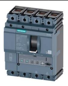
CIRCUIT BREAKER 3VA2 IEC FRAME 160 BREAKING CAPACITY CLASS M ICU=55KA @ 415 V 4POLE, LINE PROTECTION ETU330, LIG, IN=63A OVERLOAD PROTECTION IR=25A ...63A SHORT CIRCUIT PROTECTION II=1,5...12 X IN NEUTRAL PROTECTION ADJUSTABLE(OFF,100%) GROUNDFAULTPROTECTION IG=0,2... 1 X IN, TG=0,1/0,3MS CABLE CONNECTION
