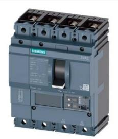
CIRCUIT BREAKER 3VA2 IEC FRAME 250 BREAKING CAPACITY CLASS M ICU=55KA @ 415 V 4POLE, LINE PROTECTION ETU550, LSI, IN=250A OVERLOAD PROTECTION IR=100A ...250A SHORT CIRCUIT PROTECTION ISD=0,6..10X IN, II=1,5..10X IN NEUTRAL PROTECTION ADJUSTABLE (OFF, UPTO 100%) BUSBAR CONNECTION
