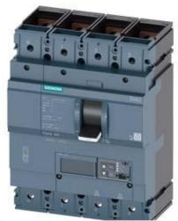
CIRCUIT BREAKER 3VA2 IEC FRAME 400 BREAKING CAPACITY CLASS M ICU=55KA @ 415 V 4-POLE, LINE PROTECTION ETU860, LSIG, IN=250A OVERLOAD PROTECTION IR=100A ...250A SHORT CIRCUIT PROTECTION ISD=0,6..10X IN, II=1,5..12X IN NEUTRAL PROTECTION ADJUSTABLE (OFF, UPTO 160%) GROUND-FAULT, SWITCHABLE IG=0,2... 1 X IN, TG=0,05-0,8MS BUSBAR CONNECTION
