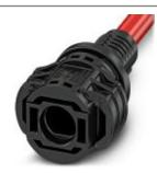
Photovoltaic connector, Range of articles: SUNCLIX, Photovoltaic connector, housing material: PPE, color: black, rated current: 20 A, Connection method: Crimp, Type of contact: Pin
