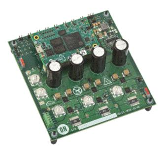
motor driver. As part of the motor development kit, the power board is compatible with the power Universal controller board enabling high-end control strategies and AI capabilities for industrial motor control. The complete kit is Strata enabled and the graphical user interface can be used to set control parameters for the motor drive.
