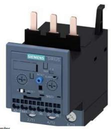
OVERLOAD RELAY 20...80 A FOR MOTOR PROTECTION SIZE S2, CLASS 5E...30E FOR MOUNTING ONTO CONTACTORS MAIN CIRCUIT: SCREW TERMINAL AUX. CIRCUIT: SPRING-TYPE TERM. MANUAL-AUTOMATIC-RESET INT. GROUND FAULT DETECTION
