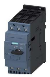
CIRCUIT BREAKER, SIZE S2, FOR STARTER COMBINATION, RATED CURRENT 36A, N-RELEASE 520A, SCREW TERMINAL, INCREASED SWITCHING CAPACITY
