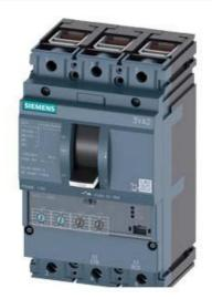
CIRCUIT BREAKER 3VA2 IEC FRAME 100 BREAKING CAPACITY CLASS L ICU=150KA @ 415 V 3POLE, LINE PROTECTION ETU330, LIG, IN=40A OVERLOAD PROTECTION IR=16A ...40A SHORT CIRCUIT PROTECTION II=1,5...12 X IN GROUNDFAULTPROTECTION IG=0,2... 1 X IN, TG=0,1/0,3MS CABLE CONNECTION
