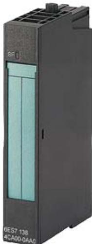
SIMATIC DP, ELECTRONIC MODULE 2 AO I HIGH FEATURE FOR ET 200S, 15 MM WIDE, CYCLE TIME PER MODULE: 0.5MS, +/- 20MA; 15 BIT + SIGN, 4 .. 20MA; 15 BIT, OPERATIONAL LIMITS +/- 0.05% WITH LED SF (GROUP FAULT)
