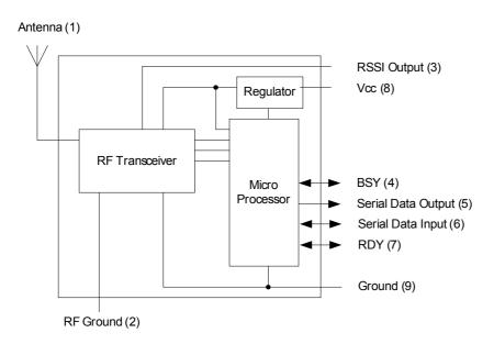
Figure 7 Easy-Radio Transceiver Block Diagram
