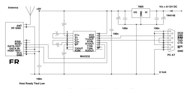
Figure 11 MAX232 Application Circuit
