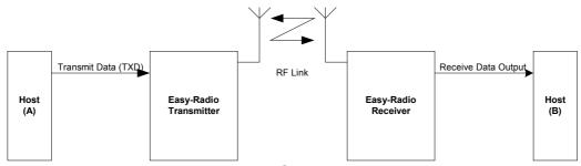
Figure 5 Typical System Block Diagram
