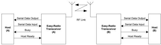
Figure 9 Typical System Block Diagram
