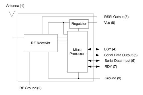
Figure 3 Easy-Radio Receiver Block Diagram
