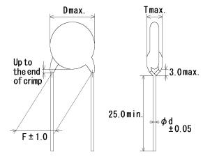
Note) The mark '\*' of Lead Style differ from lead spacing(F) and lead diameter(d).
