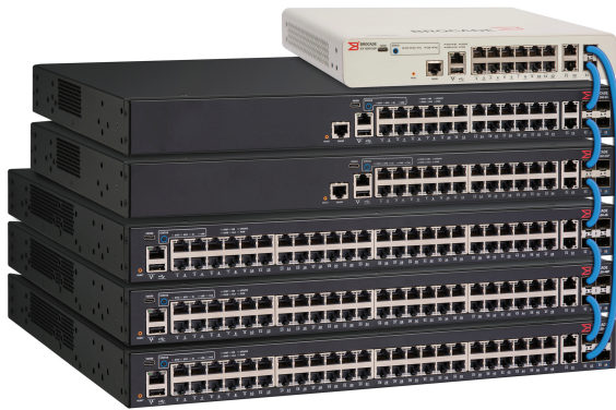
Figure 3. Up to eight Brocade ICX 7150 switches can be stacked together into a single logical switch using standard SFP+ 10 Gbps ports and copper cables or optics.
