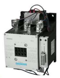
CONTACTOR, 132KW/400V/AC-3 AC(40...60HZ)/DC OPERATION UC 96-127V AUXILIARY CONTACTS 1NO+1NC 3-POLE, SIZE S10 BAR CONNECTIONS ELECTRONIC OPERATING MECHANISM WITH PLC/SIMOCODE INTERFACE AND REMAIN. LIFETIME INDICATOR
