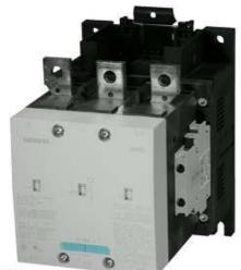
VAC. CONTACTOR, 132KW/400V/AC-3 WITHOUT COIL AUXILIARY CONTACTS 2NO+2NC 3-POLE, SIZE S10 RAIL CONNECTIONS
