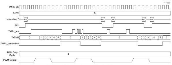
Note 1: BSF and BCF represent Bit-Set File and Bit-Clear File instructions executed by the CPU to set or clear the ON bit of TxCON. CPU execution is asynchronous to the timer clock input.
