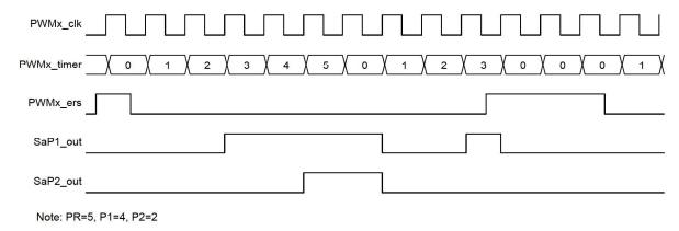
Figure 30-16. Left Aligned Mode with ERSNOW = 0
