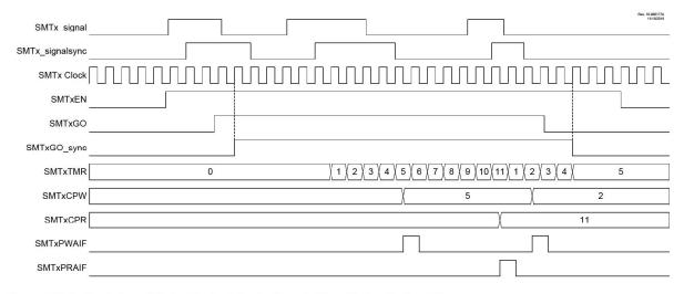
Figure 27-7. Period and Duty Cycle, Single Acquisition Mode Timing Diagram
