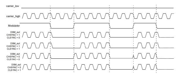
Figure 33-3. No Synchronization (CHSYNC = 0, CLSYNC = 0)
