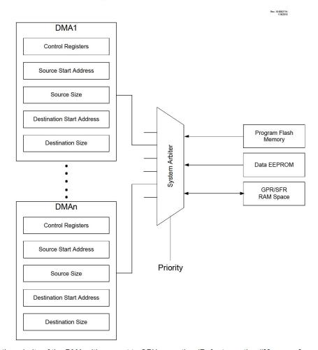
Depending on the priority of the DMA with respect to CPU execution (Refer to section "Memory Access Scheme" in the "PIC18 CPU" chapter for more information), the DMA Controller can move data through two methods:
