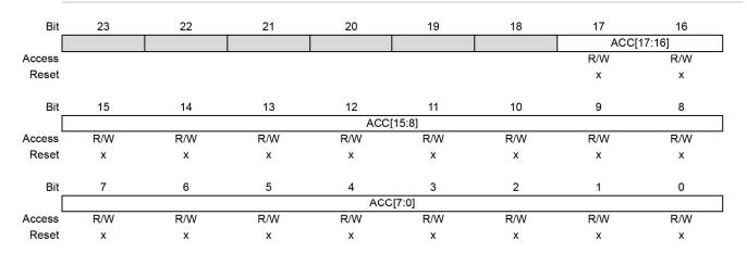
Bits 17:0 - ACC[17:0] ADC Accumulator - Signed 2's Complement
