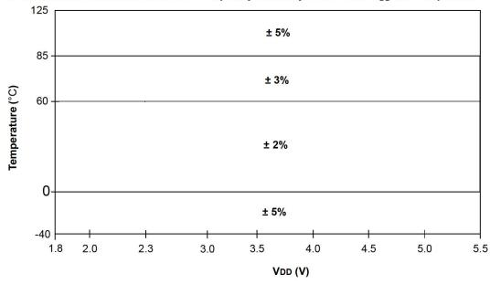
Figure 47-5. Precision Calibrated HFINTOSC Frequency Accuracy Over Device  $V_{\text{DD}}$  and Temperature
