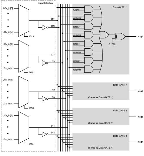
Figure 22-2. Input Data Selection and Gating
