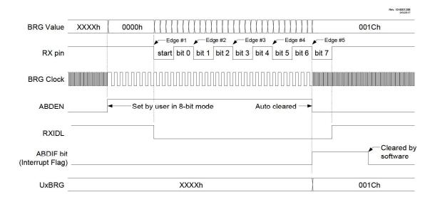
RXIDL indicates that the sync input is active. RXIDL will go low on the first falling edge and go high on the fifth rising edge
