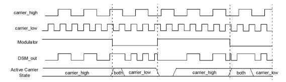
Figure 33-5. Carrier Low Synchronization (CHSYNC = 0, CLSYNC = 1)
