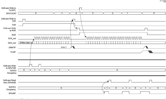
Figure 35-5. SPI Master Operation, Command+Read Data, TXR = 0, RXR = 1
