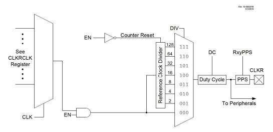
Figure 23-2. Clock Reference Timing
