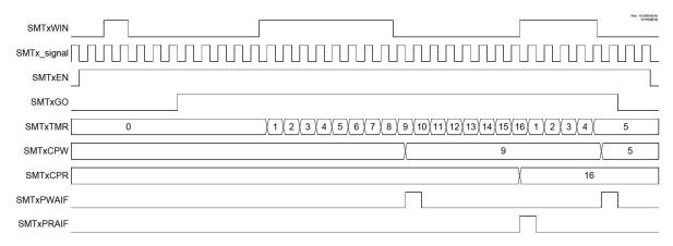
Figure 27-22. Windowed Counter Mode, Single Acquisition Timing Diagram
