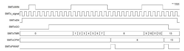
Figure 27-20. Gated Counter Mode, Single Acquisition Timing Diagram
