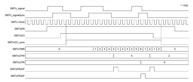
Figure 27-9. High and Low Measurement Mode, Single Acquisition Timing Diagram
