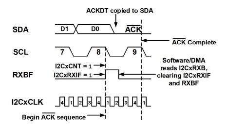
Figure 36-34. Not Acknowledge (NACK) Sequence Timing
