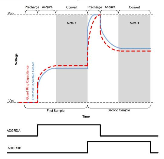
Figure 40-10. Differential CVD with Guard Ring Output Waveform
