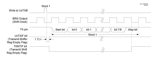
Figure 34-4. UART Asynchronous Transmission (back-to-back)
