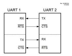
The UART receiving data asserts the  $\overline{RTS}$  output low when the input FIFO is empty. When a character is received, the  $\overline{RTS}$  output goes high until the UxRXB is read to free up both FIFO locations.
