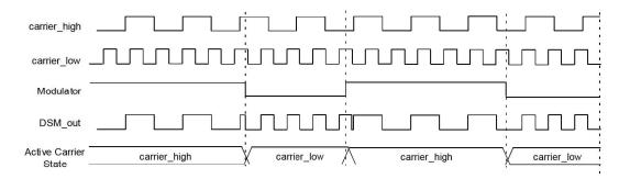
Figure 33-6. Full Synchronization (CHSYNC = 1, CLSYNC = 1)
