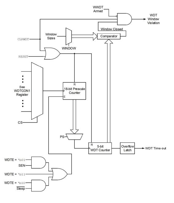
Figure 15-1. Windowed Watchdog Timer Block Diagram
