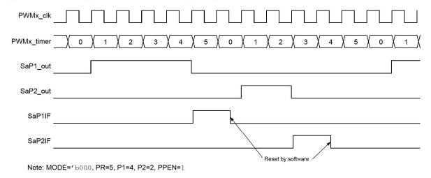
Figure 30-14. Right Aligned Push-Pull Mode Timing Diagram
