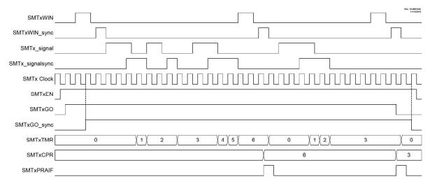
Figure 27-13. Gated Windowed Measurement Mode, Single Acquisition Timing Diagram
