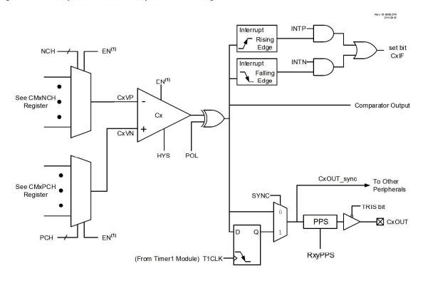
Note 1: When EN = 0, all multiplexer inputs are disconnected and the Comparator will produce a '0' at the output.
