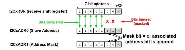
In 10-bit Address mode, I2CxADR0 and I2CxADR1, and I2CxADR2 and I2CxADR3, are combined to create two 10-bit addresses. I2CxADR0 and I2CxADR2 hold the lower eight bits of the address, while I2CxADR1 and I2CxADR3 hold the upper two bits of the address, the R/W bit, and the five-digit '11110' code assigned to the five Most Significant bits of the high address byte.
