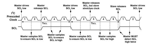
When FME is set (FME = 1), one SCL period ( $T_{SCL}$ ) is equal to four clock periods of the prescaled I2CxCLK source. In other words, the prescaled I2CxCLK source is divided by four. Using the example from above, if the HFINTOSC (4 MHz) clock source is selected, I2CxBAUD is loaded with a value of '7' and the FME bit is set, the actual SCL frequency is 125 kHz (see Equation below).
