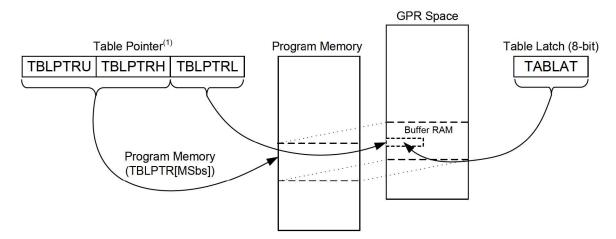
**Note 1:** During table writes the Table Pointer does not point directly to program memory. TBLPTRL actually points to an address within the buffer registers. TBLPTRU:TBLPTRH points to program memory where the entire buffer space will eventually be written with the NVM commands.
