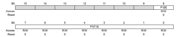
Bit 8 - P1[8] Parameter 1 Most Significant bit
