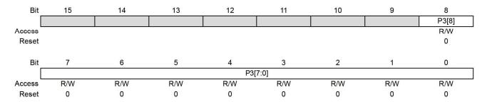
Bit 8 - P3[8] Parameter 3 Most Significant bit
