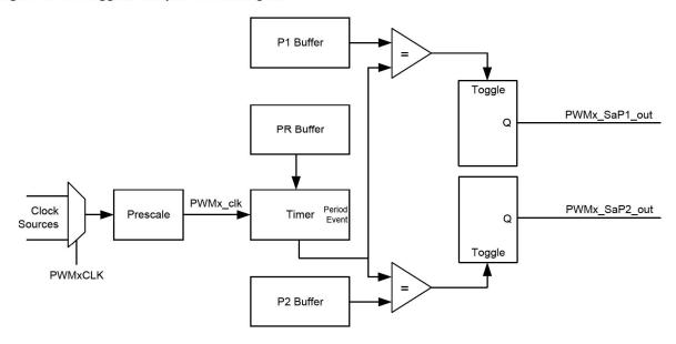
Figure 30-12. Toggled Compare Timing Diagram
