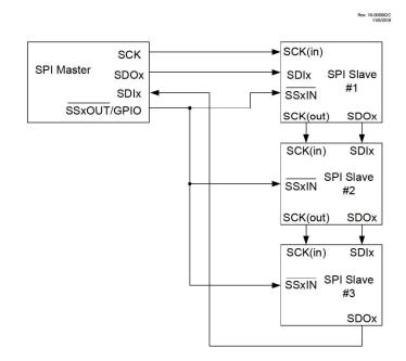
Figure 35-13. SPI Daisy-Chain Connection With Chained SCK
