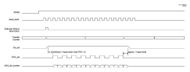
Note: 1. SDO bit number illustrates the transmitted bit number, and is not intended to imply SDO\_out tristate operation.
