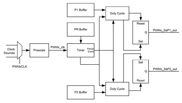
Figure 30-6. Center Aligned Timing Diagram
