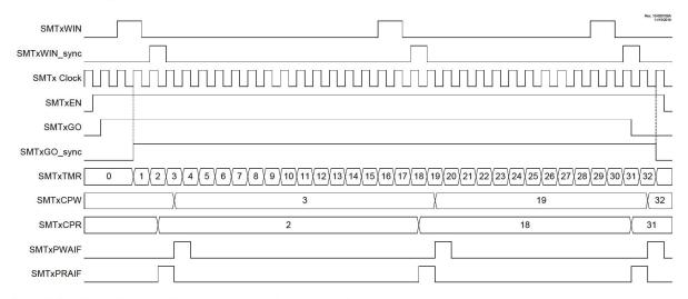
Figure 27-17. Capture Mode, Single Acquisition Timing Diagram
