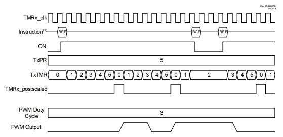
Note 1: BSF and BCF represent Bit-Set File and Bit-Clear File instructions executed by the CPU to set or clear the ON bit of TxCON. CPU execution is asynchronous to the timer clock input.
