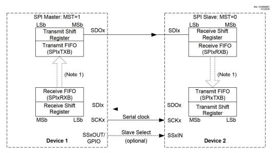
Note 1: In some modes, if the Transmit FIFO is empty, the most recently received byte of data will be transmitted.
