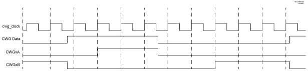
Dead-band is always initiated on the edge of the input source signal. A count of zero indicates that no dead-band is present.
