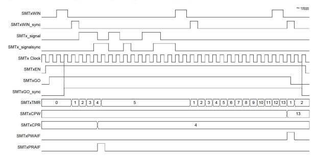
Figure 27-15. Time-of-Flight Mode, Single Acquisition Timing Diagram
