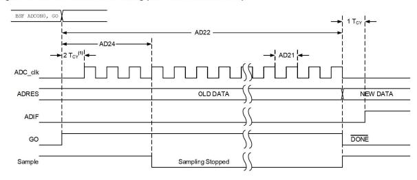
Figure 47-10. ADC Conversion Timing (ADC Clock from ADCRC)
