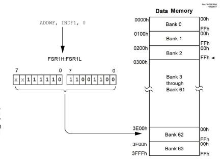
Operations on the FSRs with POSTDEC, POSTINC and PREINC affect the entire register pair; that is, rollovers of the FSRnL register from FFh to 00h carry over to the FSRnH register. On the other hand, results of these operations do not change the value of any flags in the STATUS register (e.g., Z, N, OV, etc.).
