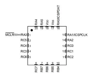
Note: It is recommended that the exposed bottom pad be connected to  $V_{SS}$ ; however, it must not be the only  $V_{SS}$ connection to the device.
