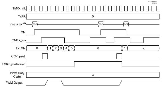
Note 1: BSF and BCF represent Bit-Set File and Bit-Clear File instructions executed by the CPU to set or clear the ON bit of TxCON. CPU execution is asynchronous to the timer clock input.
