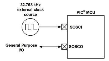
The SOSC can be enabled through one of two methods:
