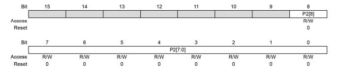
Bit 8 - P2[8] Parameter 2 Most Significant bit
