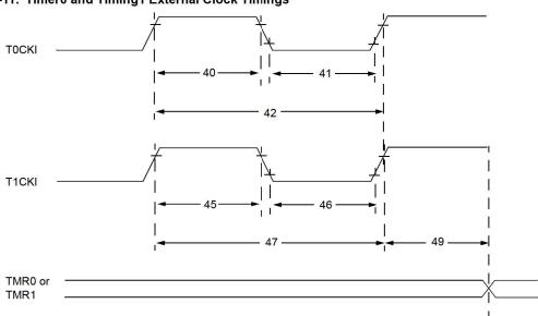
Figure 47-11. Timer0 and Timing1 External Clock Timings
