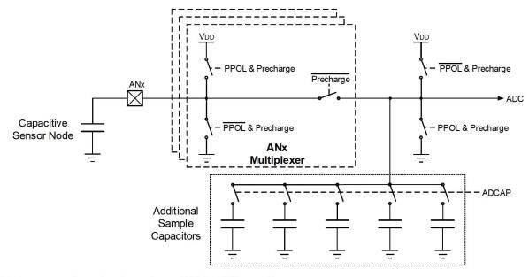
This is an example on how to configure ADC for CVD operation:
