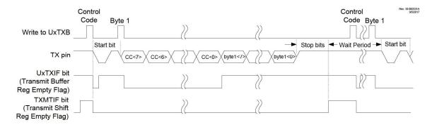
During the communication between two Control Devices, three bytes are required to be transmitted. In this case, the software must write the third byte to UxTXB as soon as UxTXIF goes true and before the output shifter becomes empty. This ensures that the three bytes of the forward frame are transmitted back-to-back without any interruption.
