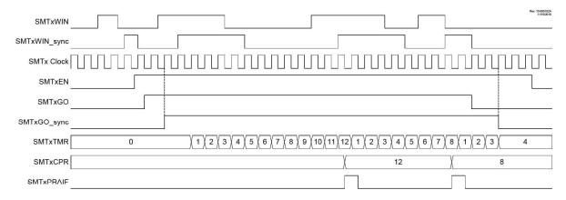
Figure 27-11. Windowed Measurement Mode, Single Acquisition Timing Diagram
