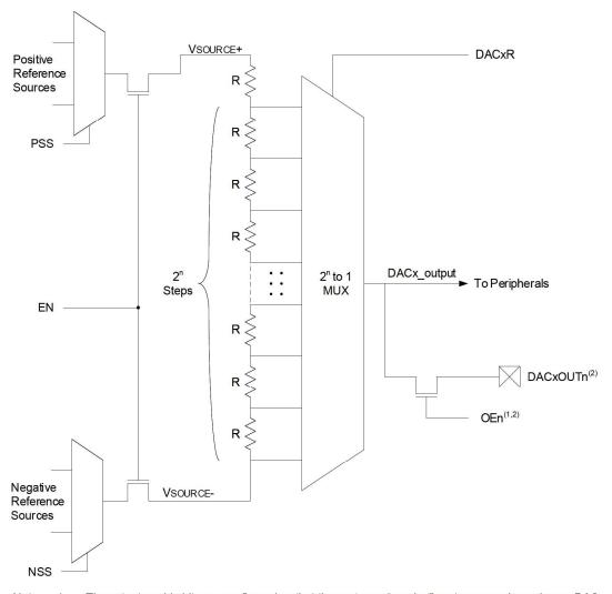
Figure 41-1. Digital-to-Analog Converter Block Diagram
