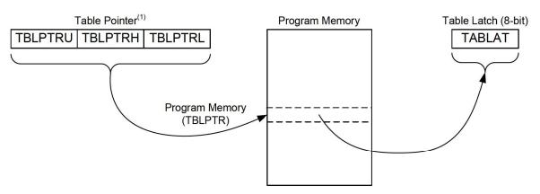
Note 1: The Table Pointer register points to a byte in program memory.
