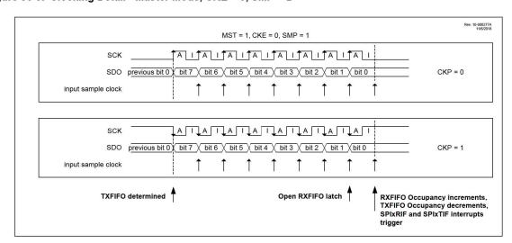
Figure 35-9. Clocking Detail - Master Mode, CKE = 0, SMP = 1
