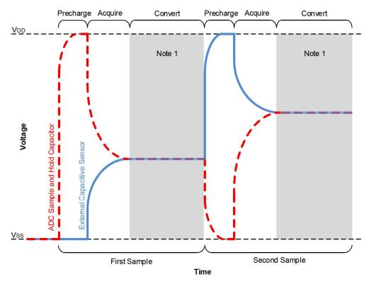
Figure 40-8. Differential CVD Measurement Waveform
