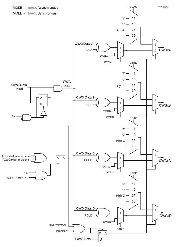
Figure 31-9. Simplified CWG Block Diagram (Output Steering Modes)
