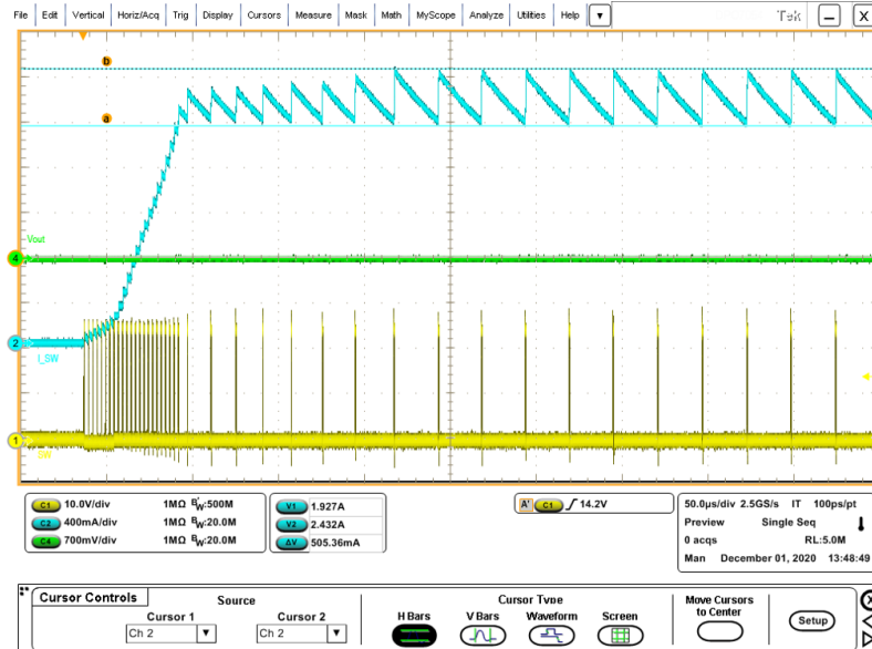
Figure 21. Soft-start procedure with VOUT shorted to GND
