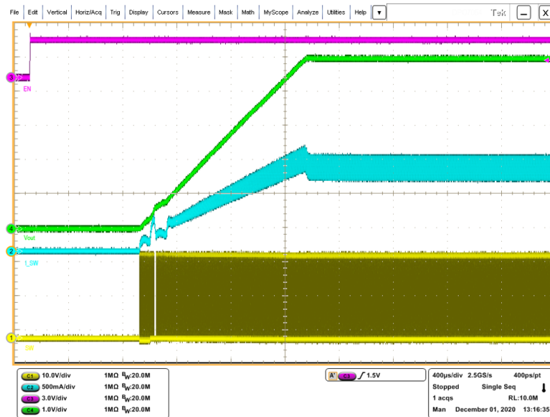
Figure 6. Soft-start phase with I_{OUT} = 1.25\text{ A}
