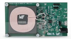
Receiver Module and LED Load Module
