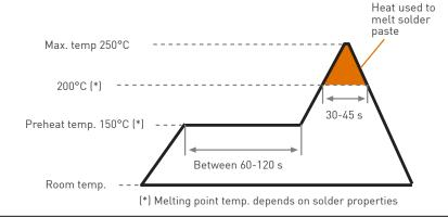
The recommended reflow profile is provided as a guideline. Optimal profile may differ due to oven type, assembly layout or other design or process variables. Customers should verify actual device performance in their specific application and reflow process. Please contact Piher if you require additional support.
