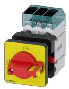
Switch disconnector 3LD3, main switch 3-polig, lu 25A operational switch at AC-23 A at 400 V 9,0 kW front mounted Base mounting with center-hole 22,5 mm knob-operated mechanism red/yellow 48 x 48 mm
