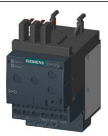
MONITORING RELAY ATTACHABLE TO CONTACTOR 3RT2. SIZE S00 BASIC, ANALOG ADJUSTABLE APPARENT CURRENT MONITORING 1.6 - 16A, 50-60 HZ, 2-PHASE SUPPLY 24-240 V AC/DC 1 CO CONTACT MONITORING FOR CURRENT OVERSHOOT/UNDERSHOOT PHASE FAILURE, WIRE BREAK WITH OR W/O ERROR LOG ON-DELAY 0-60 S SPURIOUS PEAK SUPPR.0-30 S SWITCHING HYSTERESIS 6% SPRING-LOADED CONNECTION
