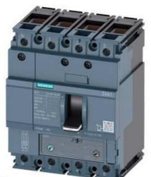
CIRCUIT BREAKER 3VA1 IEC FRAME 160 BREAKING CAPACITY CLASS S ICU=36KA @ 415 V 4-POLE, LINE PROTECTION TM240, ATAM, IN=63A OVERLOAD PROTECTION IR=44,1A ...63A SHORT CIRCUIT PROTECTION II=5...10 X IN NEUTRAL PROTECTION 100% CABLE CONNECTION
