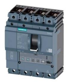
CIRCUIT BREAKER 3VA2 IEC FRAME 160 BREAKING CAPACITY CLASS H ICU=85KA @ 415 V 4POLE, LINE PROTECTION ETU350, LSI, IN=63A OVERLOAD PROTECTION IR=25A ...63A SHORT CIRCUIT PROTECTION ISD=1,5... 10 X IR, II=12 X IN NEUTRAL PROTECTION ADJUSTABLE(OFF,100%) BUSBAR CONNECTION
