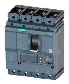
CIRCUIT BREAKER 3VA2 IEC FRAME 250 BREAKING CAPACITY CLASS L ICU=150KA @ 415 V 4POLE, LINE PROTECTION ETU850, LSI, IN=160A OVERLOAD PROTECTION IR=64A ...160A SHORT CIRCUIT PROTECTION ISD=0,6..10X IN, II=1,5..12X IN NEUTRAL PROTECTION ADJUSTABLE (OFF, UPTO 160%) BUSBAR CONNECTION
