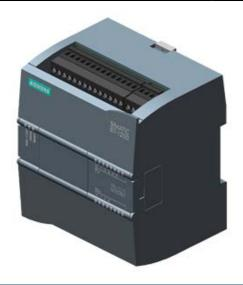
SIMATIC S7-1200, CPU 1211C, COMPACT CPU, AC/DC/RELAY, ONBOARD I/O: 6 DI 24V DC; 4 DO RELAY 2A; 2 AI 0 - 10V DC, POWER SUPPLY: AC 85 - 264 V AC AT 47 - 63 HZ, PROGRAM/DATA MEMORY: 30 KB
