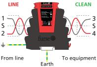
ESP SL RS485 installed in series
