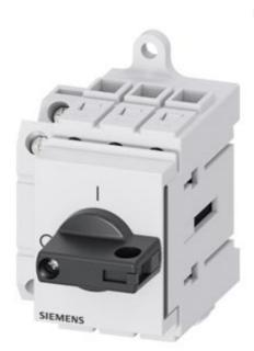
Switch disconnector 3LD3, main switch 3-polig, lu 40A operational switch at AC-23 A at 400 V 15,0 kW Distribution board mounting Base mounting with knob-operated mechanism black with auxiliary 1NO+1NC
