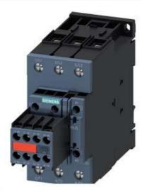
CONTACTOR,AC3:22KW/400V, 2NO+2NC, 230V AC 50HZ, 3-POLE, SIZE S2, SCREW TERMINAL, AUXILIARY CONTACT INSEPARABLE
