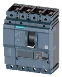
CIRCUIT BREAKER 3VA2 IEC FRAME 160 BREAKING CAPACITY CLASS L ICU=150KA @ 415 V 4POLE, LINE PROTECTION ETU850, LSI, IN=40A OVERLOAD PROTECTION IR=16A ...40A SHORT CIRCUIT PROTECTION ISD=0,6..10X IN, II=1,5..12X IN NEUTRAL PROTECTION ADJUSTABLE (OFF, UPTO 160%) BUSBAR CONNECTION
