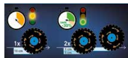
Patented cutting depth indicator
