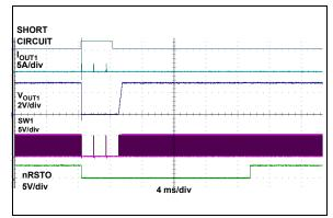
**FIGURE 2-17:** Output Short Circuit on V<sub>OUT1</sub>.
