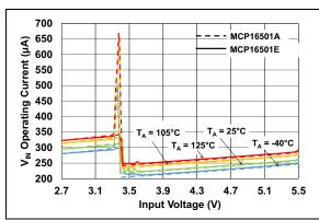
**FIGURE 2-2:**  $V_{IN}$  Quiescent Current vs. Input Voltage and Temperature – Low-Power Mode (LPM = PWRHLD = High).
