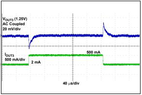
**FIGURE 2-16:** Buck3 Transient Response (Active Mode,  $V_{OUT3} = 1.25V$ ).
