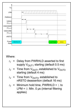
FIGURE 4-9: Start-up Sequence Exiting Hibernate Mode Timing Diagram.
