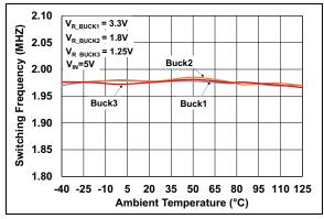
FIGURE 2-7: Switching Frequency vs.
