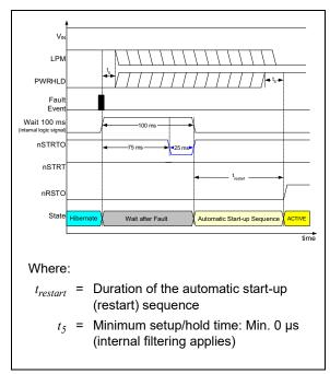
FIGURE 4-10: Automatic Wake-Up Pulse Generation Timing Diagram (Fault during Hibernate).
