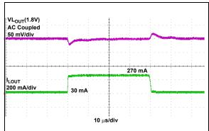
FIGURE 2-18: LDO Load Transient Response.
