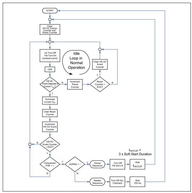
FIGURE 5-1: Hiccup Mode Protection Flowchart.
