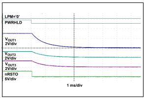
FIGURE 2-14: PWRHLD Shutdown Sequence.
