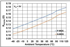
**FIGURE 2-9:** MOSFET  $R_{DS(ON)}$  vs. Temperature.
