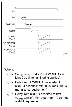
**FIGURE 4-7:** Power-Down (Shutdown) Sequence Timing Diagram.
