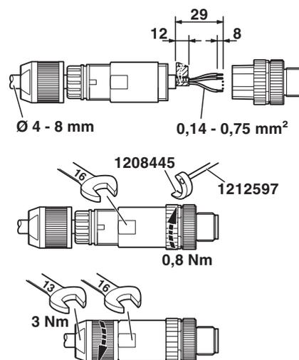
Slide the pressure nut and sleeve housing along the cable, strip the cable, shorten the shield, strip the single wires, connect the wires, in the case of a straight sleeve housing gently twist the wires together, stick the shielding foil around the shortened shield, in the case of a cable outside diameter < 6 mm stick an additional shielding foil around the wire pack, screw the sleeve housing to the plug insert, screw the pressure nut tight.
