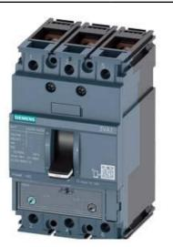
CIRCUIT BREAKER 3VA1 IEC FRAME 160 BREAKING CAPACITY CLASS S ICU=36KA @ 415 V 3-POLE, LINE PROTECTION TM240, ATAM, IN=25A OVERLOAD PROTECTION IR=17,5A ...25A SHORT CIRCUIT PROTECTION II=6,4...12,8 X IN BUSBAR CONNECTION
