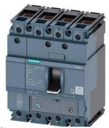
CIRCUIT BREAKER 3VA1 IEC FRAME 160 BREAKING CAPACITY CLASS M ICU=55KA @ 415 V 4-POLE, LINE PROTECTION TM240, ATAM, IN=32A OVERLOAD PROTECTION IR=22,4A ...32A SHORT CIRCUIT PROTECTION II=5...10 X IN NEUTRAL PROTECTION 100% CABLE CONNECTION
