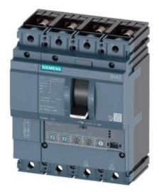
CIRCUIT BREAKER 3VA2 IEC FRAME 100 BREAKING CAPACITY CLASS H ICU=85KA @ 415 V 4POLE, LINE PROTECTION ETU350, LSI, IN=40A OVERLOAD PROTECTION IR=16A ...40A SHORT CIRCUIT PROTECTION ISD=1,5... 10 X IR, II=12 X IN NEUTRAL PROTECTION ADJUSTABLE(OFF,100%) BUSBAR CONNECTION
