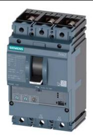
CIRCUIT BREAKER 3VA2 IEC FRAME 100 BREAKING CAPACITY CLASS C ICU=110KA @ 415 V 3POLE, LINE PROTECTION ETU320, LI, IN=40A OVERLOAD PROTECTION IR=16A ...40A SHORT CIRCUIT PROTECTION II=12 X IN BUSBAR CONNECTION
