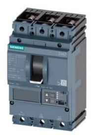
CIRCUIT BREAKER 3VA2 IEC FRAME 250 BREAKING CAPACITY CLASS H ICU=85KA @ 415 V 3POLE, LINE PROTECTION ETU860, LSIG, IN=250A OVERLOAD PROTECTION IR=100A ...250A SHORT CIRCUIT PROTECTION ISD=0,6..10X IN, II=1,5..10X IN NEUTRAL PROTECTION OPTIONAL WITH EXT. CT,UPTO 160% GROUNDFAULT, SWITCHABLE IG=0,2... 1 X IN, TG=0,050,8MS BUSBAR CONNECTION
