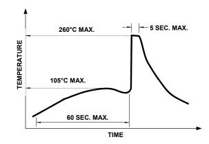
**NOTE:** Refers to measurements with thermocouple mounted at the bottom of the PCB.
