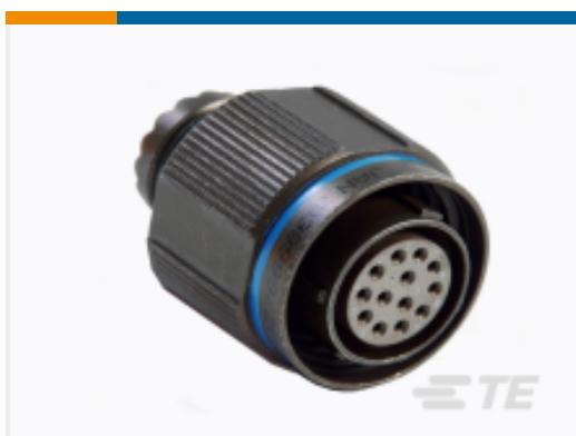
TE Part #YDTS26W15-15SNV001 D38999: Straight Plug, 15-15 Insert
