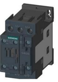
CONTACTOR, AC-3, 5.5KW/400V, 1NO+1NC, AC 24V 50HZ, 3-POLE, SZ S0 SCREW TERMINAL VERTICAL MOUNTING POSITION
