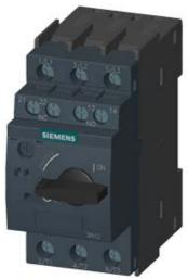
CIRCUIT-BREAKER SZ S0, FOR TRANSFORMER PROT. A-RELEASE 16...22A, N-RELEASE 364A, SCREW CONNECTION, STANDARD SW. CAPACITY W. TRANSVERSE AUX. SWITCH 1NO+1NC
