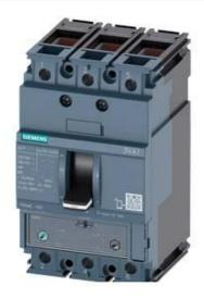
CIRCUIT BREAKER 3VA1 IEC FRAME 160 BREAKING CAPACITY CLASS M ICU=55KA @ 415 V 3-POLE, LINE PROTECTION TM240, ATAM, IN=50A OVERLOAD PROTECTION IR=35A ...50A SHORT CIRCUIT PROTECTION II=5...10 X IN CABLE CONNECTION
