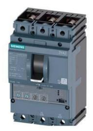
CIRCUIT BREAKER 3VA2 IEC FRAME 100 BREAKING CAPACITY CLASS L ICU=150KA @ 415 V 3POLE, LINE PROTECTION ETU330, LIG, IN=100A OVERLOAD PROTECTION IR=40A ...100A SHORT CIRCUIT PROTECTION II=1,5...12 X IN GROUNDFAULTPROTECTION IG=0,2... 1 X IN, TG=0,1/0,3MS BUSBAR CONNECTION
