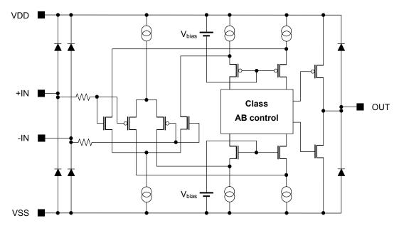
Figure 1. Simplified Schematic
