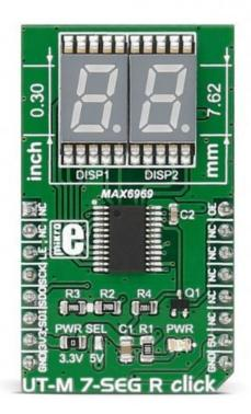
**UT-M 7-SEG R click** carries two SMD ultra thin LED 7-SEG <u>displays</u> and the <u>MAX6969</u> constant-current LED driver from Maxim Integrated. The click is designed to run on either 3.3V or 5V power supply. It communicates with the target microcontroller over SPI interface.
