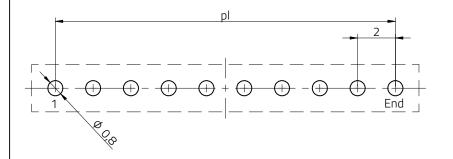
Recommended PCB Layout General tolerance ±0.05
