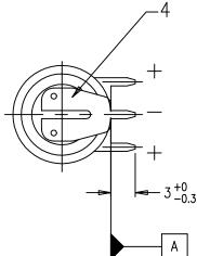
Note: 1)No welding onto the groove
